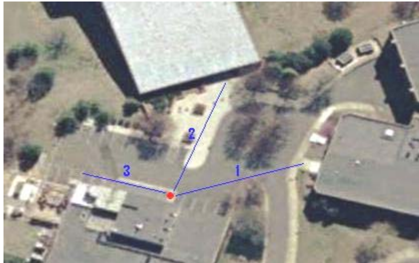
Figure 1. Environment used for reverberant decay measurements. The red dot represents the loudspeaker location and the radial lines represent the microphone ranges. Radial line three intersects a protruding wall.
